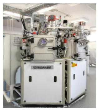
The SAF25/50 multifunctional R&D cluster tool. Dimensions (LxWxH) 3x3x2 m. Weight 2800 kg. Installed power 50 kW Cooling water 2.7 m<sup>3</sup>/h
